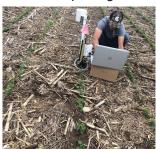
Water content below the root zone can be used to determine when to irrigate:
